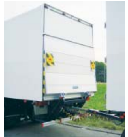
DH-LMK adapted for trailer-coupling, with 3-piece bumper bar
