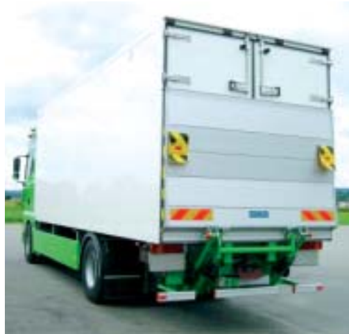
DH-LM 1500 kg with aluminium platform and 3-piece bumper bar
