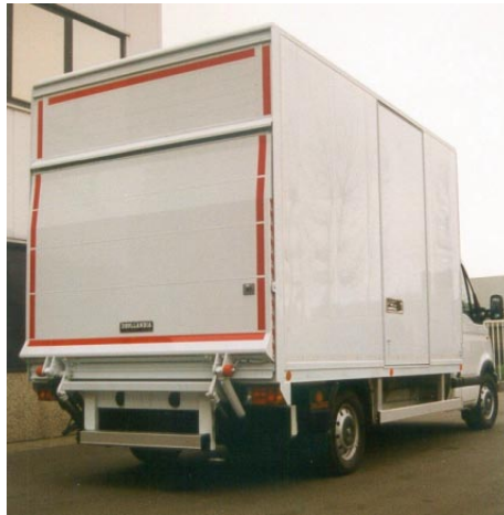
DH-LSP 3 mounted behind the spring hangars
