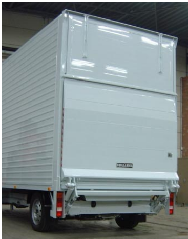
DH-LSP 6 mounted besides the springs hangars
