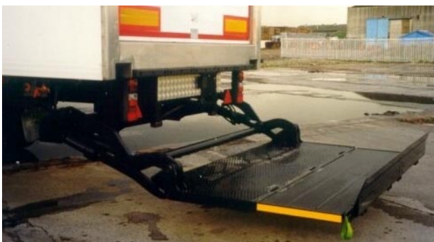
DH-SK with 1500 mm folding steel / alu platform & front loading ramps
