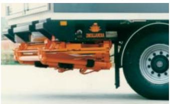
The slider lift type DH-SO5 is equipped with a compact frame construction, which fits extremely well for vehicles with minimal overhang behind the mud-guard.
