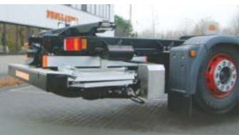
The slider lift DH-SO81 is derived from the DH-SO7, and is delivered with a 3-piece platform: a front beam in steel followed by 2 aluminium sections which are double folded and rest on the lift arms in the stowed driving position.
