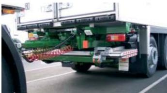
The slider lift DH-SO7 is equipped with a special frame construction and a compact hydraulic power pack. This configuration allows a lift with a wide arm centre to mount beside the spring hangards of the vehicle on quite narrow vehicle bodies (from 2150mm width onwards).
